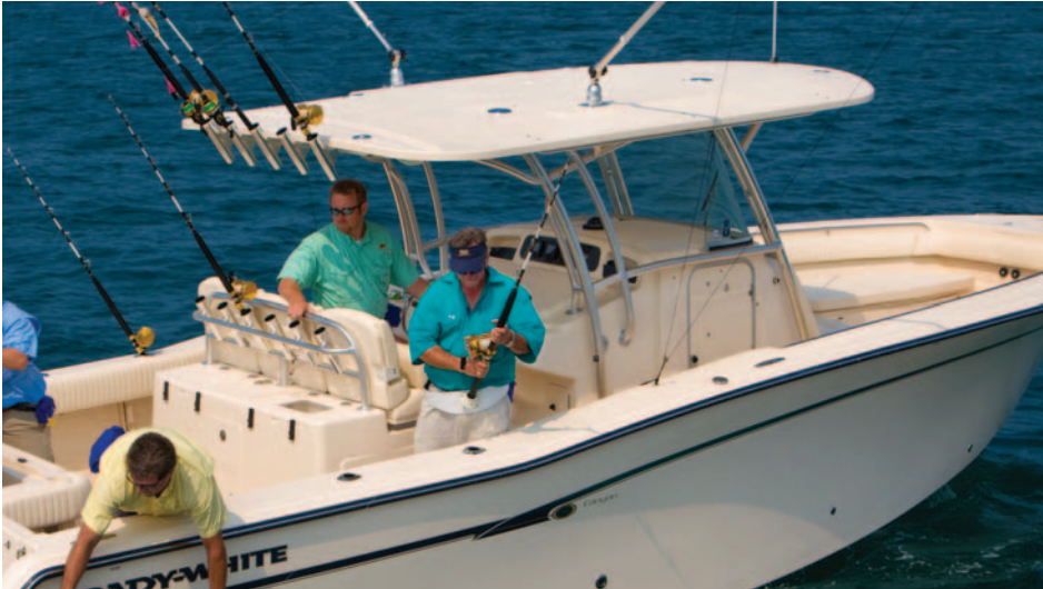
Fiberglass T-top with spreader lights (271, 283, 306, 336; standard on 376)
