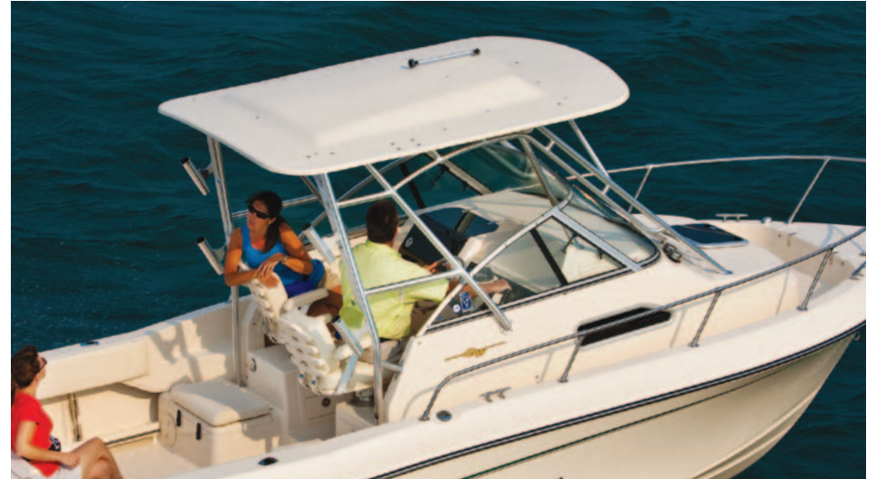
Hardtop with radio box and spreader lights (208, 226, 228, 232, 258; standard on 290, 300, 330, 370)
