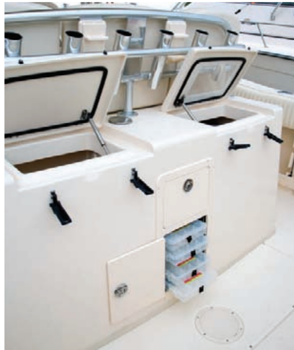
Rigging station with freshwater washdown, 104-qt. cooler, tackle drawers, storage, rod holders and knife & pliers holder
