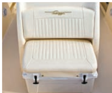
72-qt. (68 l) removable cooler seat forward (cooler upgrade shown)
