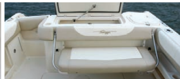
Aft fold away bench seating, 185-qt. insulated fish box, and 128-qt. cooler (32-gal. livewell optional)
