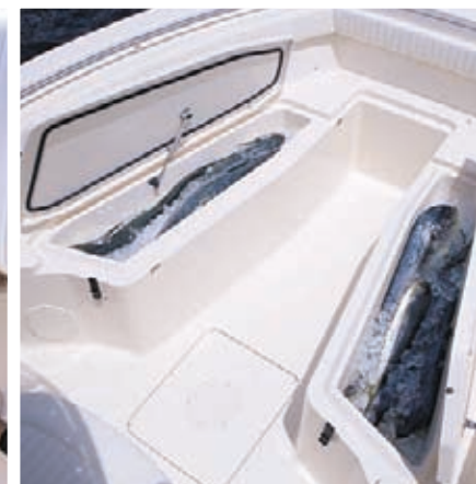
Bow fish boxes convert to bow seats (optional casting platform insert available)
