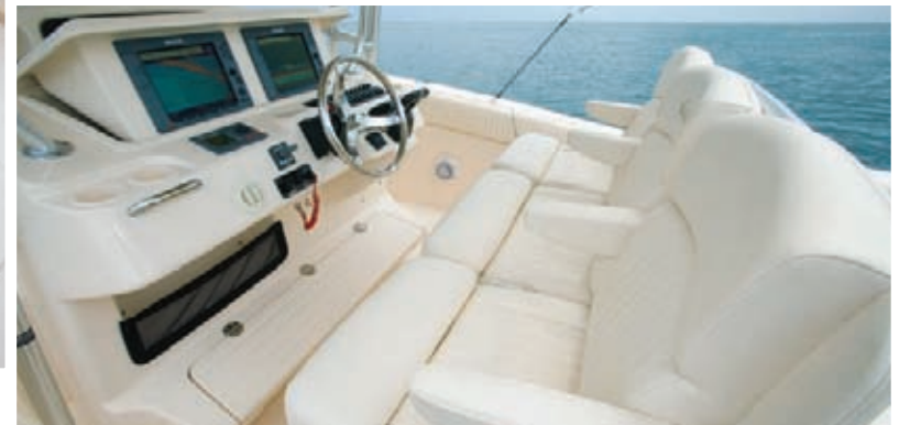
Center helm lean bar with three deluxe sliding seats and footrest, electromechanically operated lockable electronics enclosure
