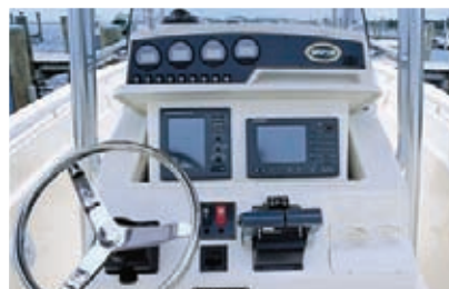
Helm console with electromechanically operated lockable electronics enclosure
