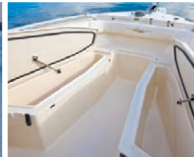
101-qt. (96 l) port and starboard forward insulated fish boxes w/ob drain. Access to bow at deck level.
