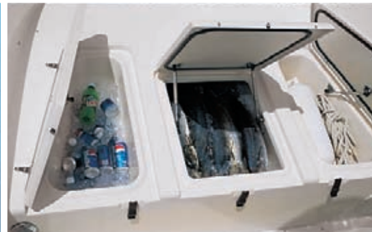
Insulated bow fish boxes with overboard drains
