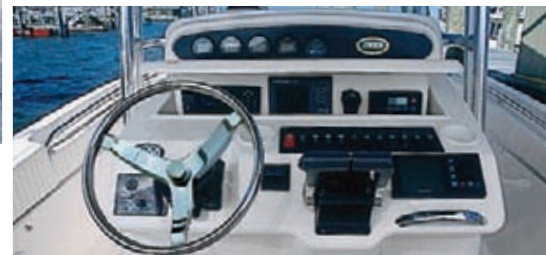
Helm console with electromechanically operated lockable electronics enclosure
