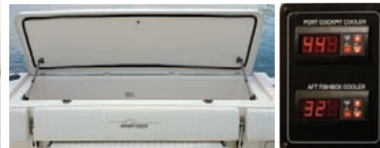
291-qt. aft deck refrigerator/freezer fish box (shown) along with 55-qt. refrigerator/freezer aft helm port box (not shown), both controlled by digital thermostat. Chill coils are located in the walls of foam insulated boxes, increasing efficiency and greatly reducing the need for ice. Coil configuration and overboard drains keep boxes clean, open and easy to maintain.
