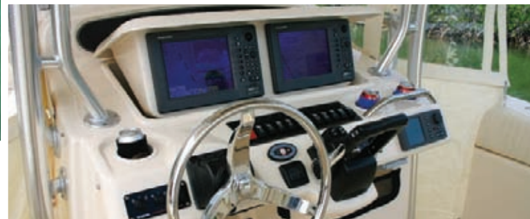
Helm console with electromechanically operated lockable electronics enclosure
