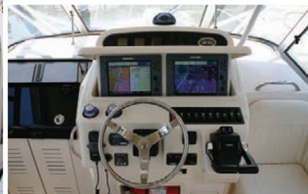
Helm station with electromechanically operated lockable electronics enclosure
