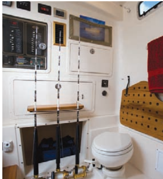
Lockable console interior with stand up head, shower, sink, rod storage, bulk storage and electrical access
