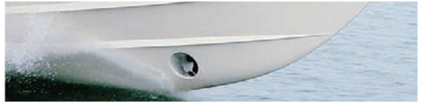
▲ Bow thruster (290, 300, 305, 306, 307, 330, 336); standard on 360, 366
