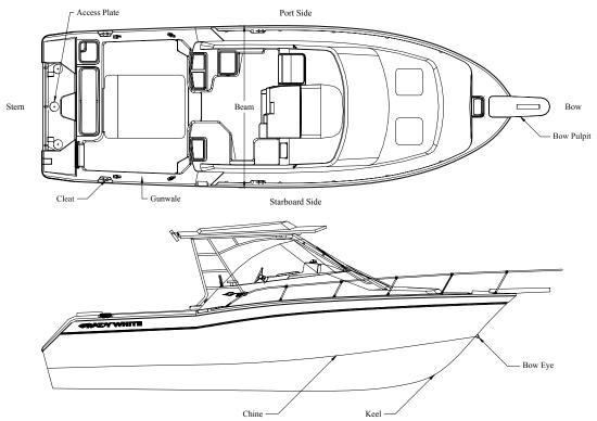
**Abeam** - a line perpendicular to a boat's keel
