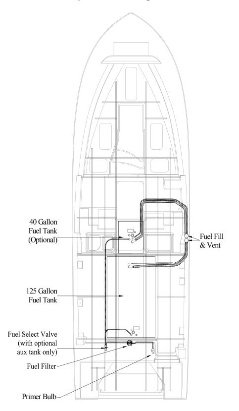
Fuel System – Dual 40 Gallon Fuel Tank Fuel Fill (Optional) & Vent 125 Gallon Fuel Tank ,0 ,0 Fuel Select Valve (with optional 匓 0 aux tank only) Fuel Filters Primer Bulbs
