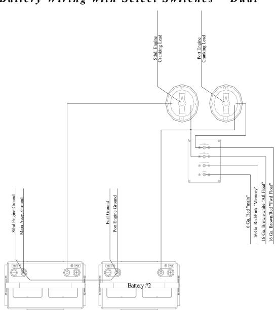
Battery Wiring with Select Switches – Dual
