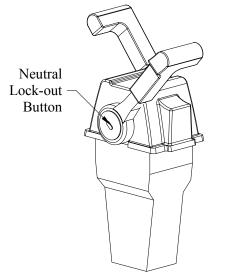
Reverse the shift mechanism to stop a boat that is moving forward. This change in direction will provide a "braking action" and slow the boat.
