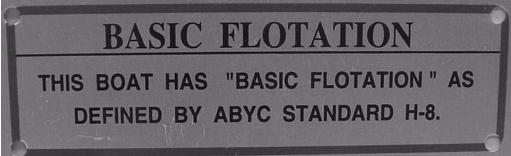
This label means that Grady-White has designed and built your boat to the ABYC basic flotation standard H-8. Basic flotation is defined as having enough foam in the boat to create buoyancy and prevent sinking under swamped conditions.
