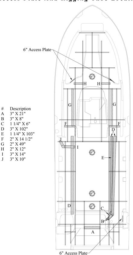
Access Plate And Rigging Tube Location
