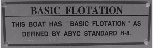
This label means that Grady-White has designed and built your boat to the ABYC basic flotation standard H-8. Basic flotation is defined as having enough foam in the boat to create buoyancy and prevent sinking under swamped conditions.
