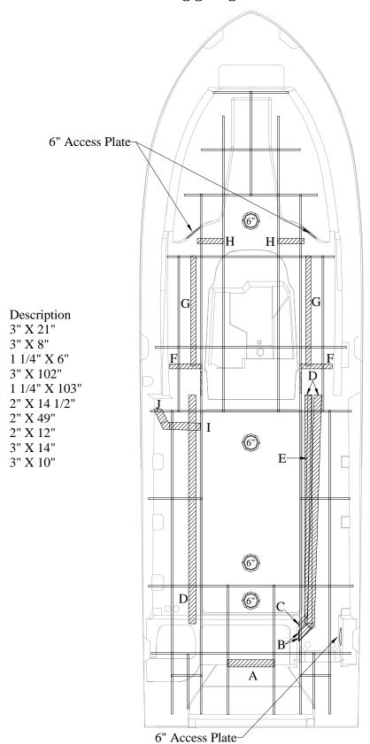
Access Plate And Rigging Tube Location
