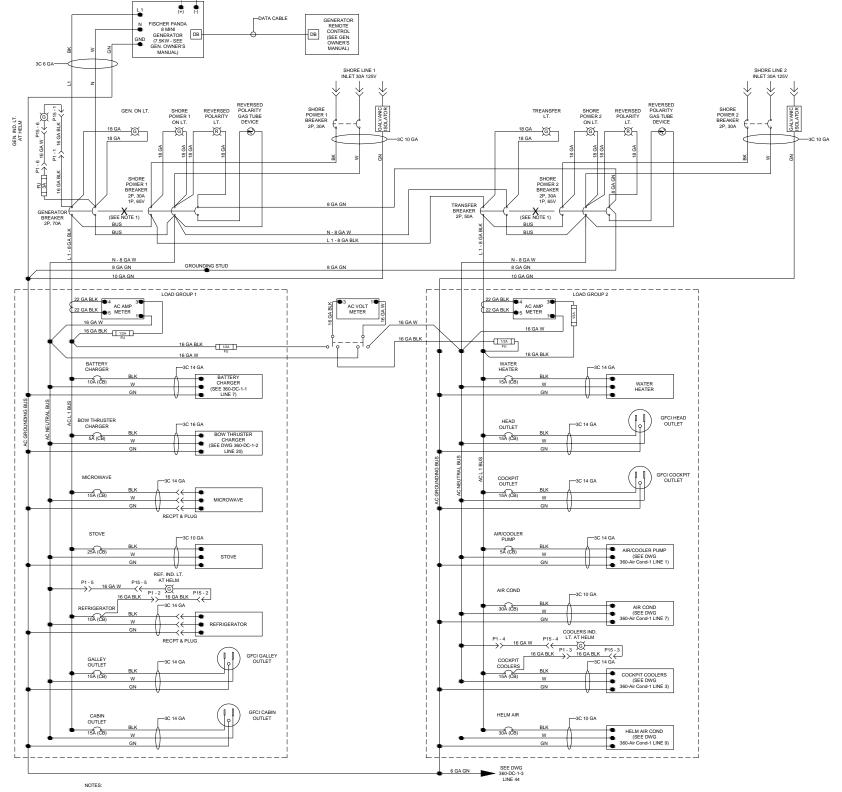
1) "X" INDICATES A MECHANICAL INTERLOCK TO PREVENT SIMULTANEOUS CLOSURE OF CIRCUIT BREAKERS.
