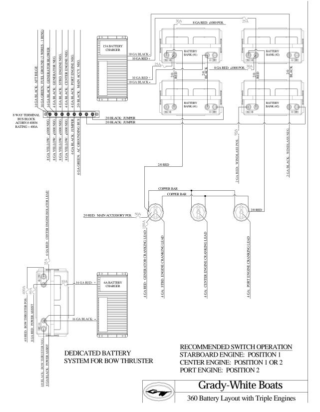
Battery Wiring With Select Switches (triple engines)
