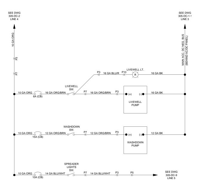
12 Volt DC Cockpit Switch Panel Diagram
