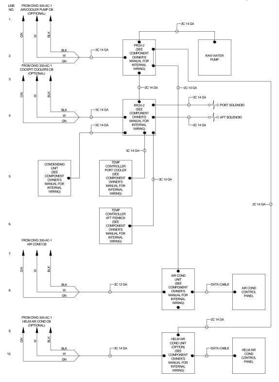
120V Air Con. & Coolers One-line Diagram
