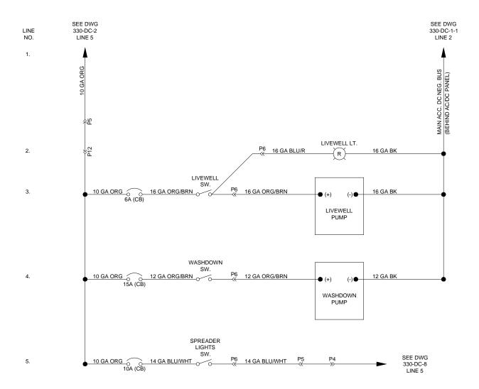
12 Volt DC Cockpit Switch Panel Diagram
