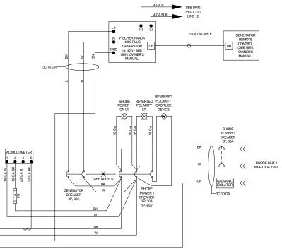
NOTES: 1) 'X' INDICATES A MECHANICAL INTERLOCK TO PREVENT SIMULTANEOUS CLOSURE OF CIRCUIT BREAKERS. 2) - A O- INDICATES MULTI-CONDUCTOR CABLE
