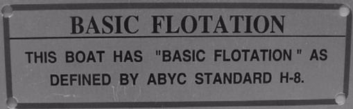
This label means that Grady-White has designed and built your boat to the ABYC standard H-8, buoyancy in the event of swamping. Basic flotation is defined as having enough foam in the boat to create buoyancy and prevent sinking under swamped conditions.
