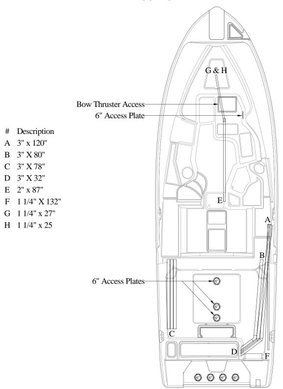
Access Plate And Rigging Tube Locations
