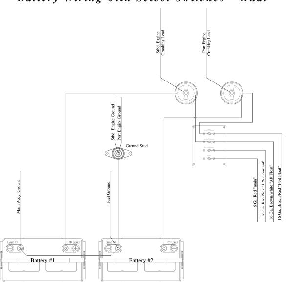
Battery Wiring with Select Switches - Dual
