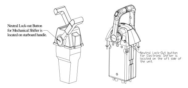
Reverse the shift mechanism to stop a boat that is moving forward. This change in direction will provide a "braking action" and slow the boat.
