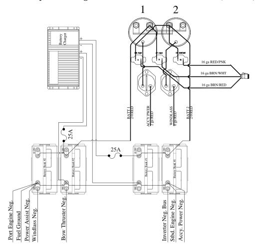
Battery Wiring with Select Switches (Dual)
