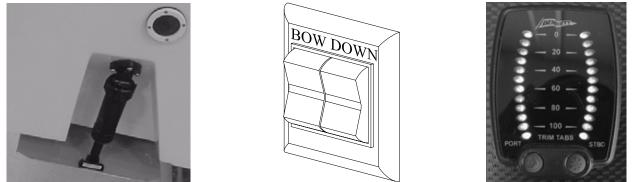
Trim tabs are also useful in correcting a port or starboard running list. If the boat is listing to the port side, press the starboard trim tab switch toward "bow down". Press the port trim tab switch toward "bow down" to correct a starboard list. This will tend to lower the bow by pulling the higher side to a level position.
