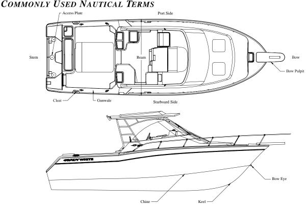
Abeam - a line perpendicular to a boat's keel
