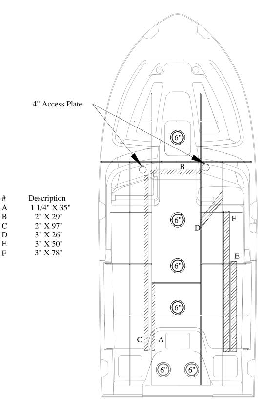
Access Plate And Rigging Tube Locations
