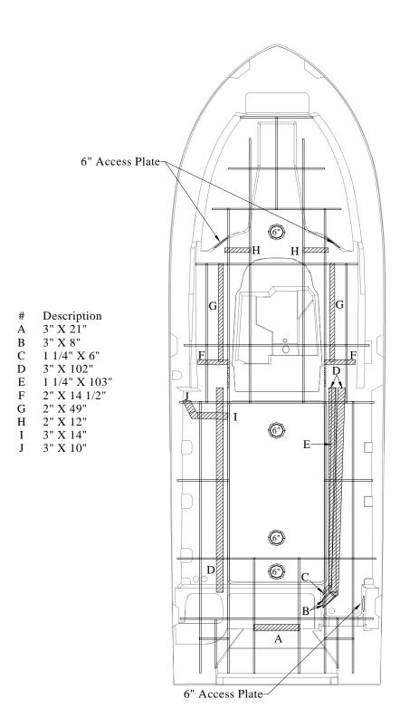
Access Plate And Rigging Tube Location
