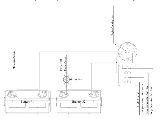
Battery Wiring with Select Switch – Single
