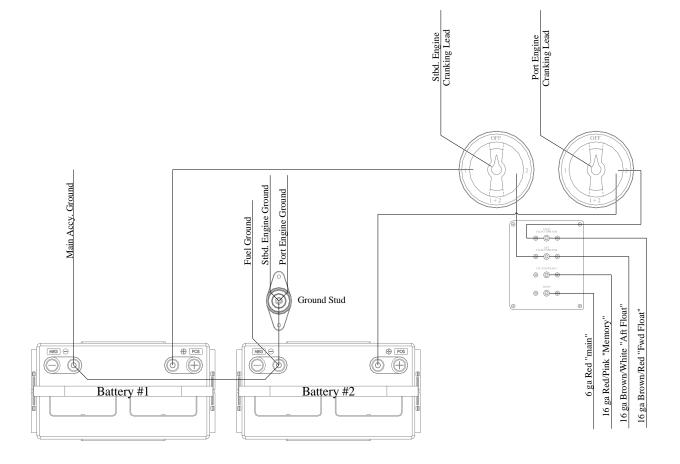
Battery Wiring with Select Switches - Twin
