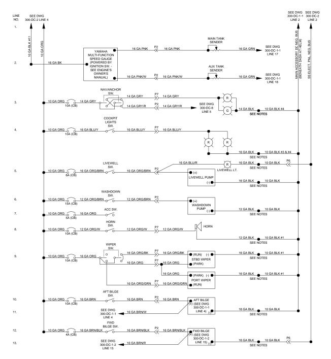
12 Volt DC Cockpit Switch Panel Diagram
