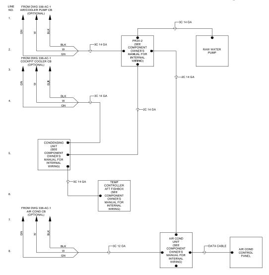
120V Air Con. & Cooler One-line Diagram
