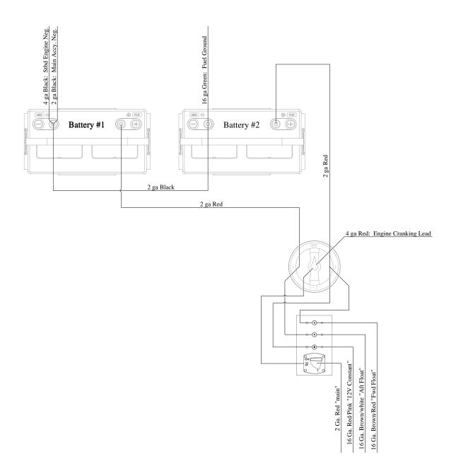
Battery Wiring with Select Switches (Dual)
