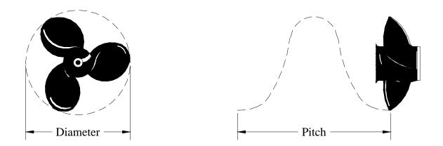
Diameter and pitch are the two basic dimensions of a propeller. Diameter is the distance across the circle made by the blade tips as the propeller rotates. Pitch is the theoretical (not accounting for slippage) forward distance the propeller would move in one revolution. An example of a propeller dimension would be 14 X 17 for a propeller having a diameter of 14" and a pitch of 17".
