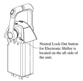
Reverse the shift mechanism to stop a boat that is moving forward. This change in direction will provide a "braking action" and slow the boat.
