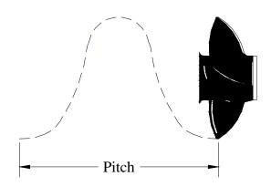
Diameter and pitch are the two basic dimensions of a propeller. Diameter is the distance across the circle made by the blade tips as the propeller rotates. Pitch is the theoretical (not accounting for slippage) forward distance the propeller would move in one revolution. An example of a propeller dimension would be 14 X 17 for a propeller having a diameter of 14" and a pitch of 17".
