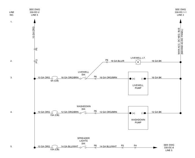
12 Volt DC Cockpit Switch Panel Diagram
