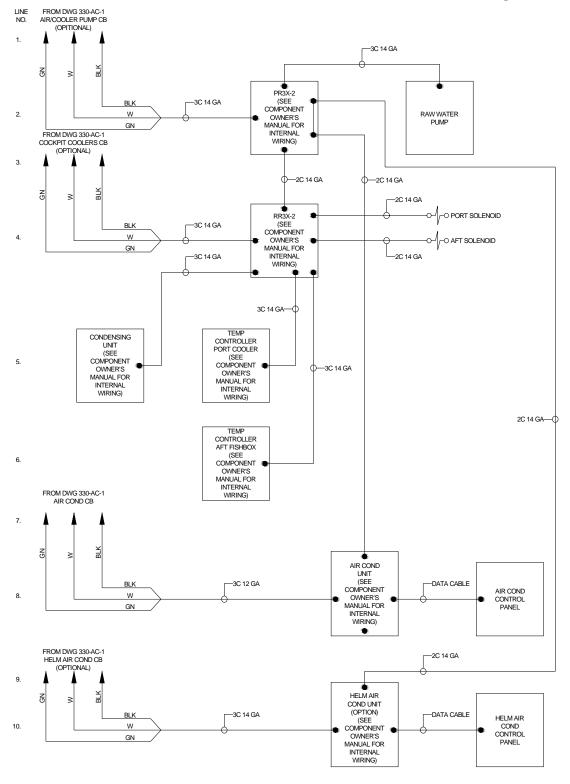
120V Air Con. & Coolers One-line Diagram
