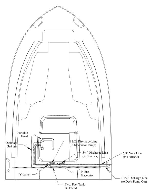
Y-valve is mounted horizontal on fwd. fuel tank bulkhead. It can be accessed through the 6" access plate, near floor level, on the aft console wall.
