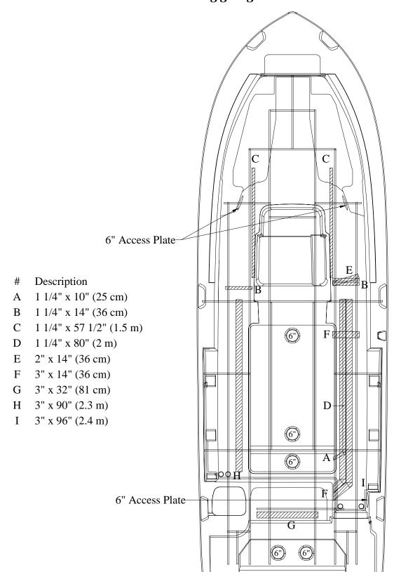
Access Plate And Rigging Tube Location
