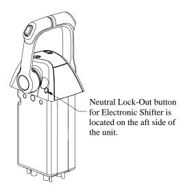
Reverse the shift mechanism to stop a boat that is moving forward. This change in direction will provide a "braking action" and slow the boat. Boats with three outboard engines are equipped
