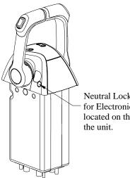
Neutral Lock-Out button for Electronic Shifter is located on the aft side of
