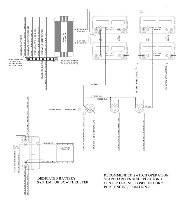
Battery Wiring With Select Switches (dual engines)
