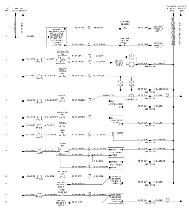
12 Volt DC Cockpit Switch Panel Diagram
