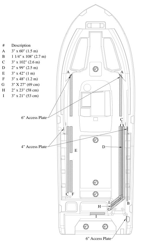
Access Plate And Rigging Tube Location
