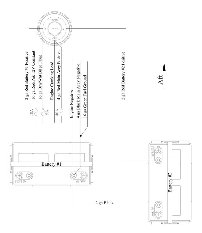
Battery Wiring with Select Switch
