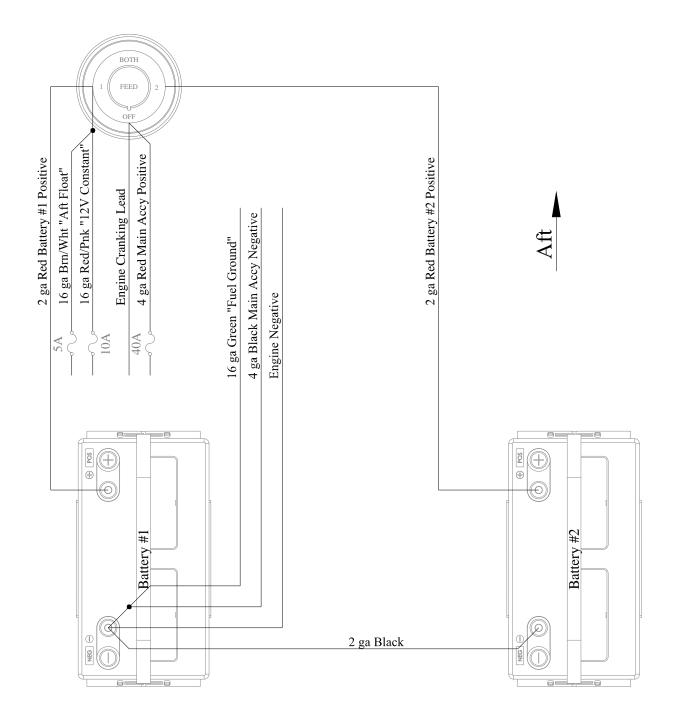
Battery Wiring with Select Switch
