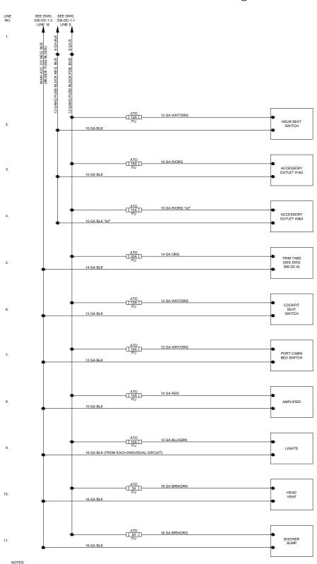
12V DC Fuse Block Diagram
