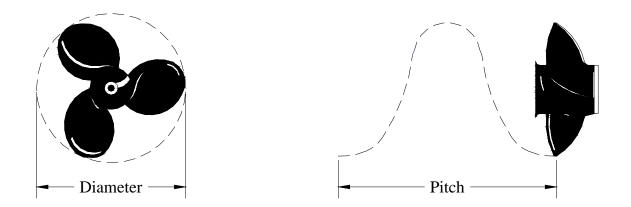
Diameter and pitch are the two basic dimensions of a propeller. Diameter is the distance across the circle made by the blade tips as the propeller rotates. Pitch is the theoretical (not accounting for slippage) forward distance the propeller would move in one revolution. An example of a propeller dimension would be 14 X 17 for a propeller having a diameter of 14" (35.6cm) and a pitch of 17" (43.8cm).
