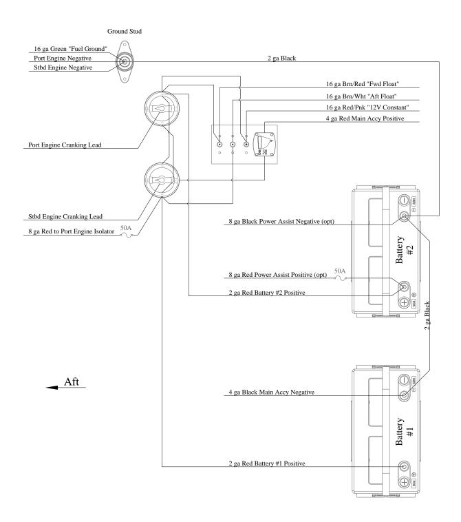
NOTE: 50A engine isolator fuse changes to 100A MRCB if the boat is equipped with V6 engines.
