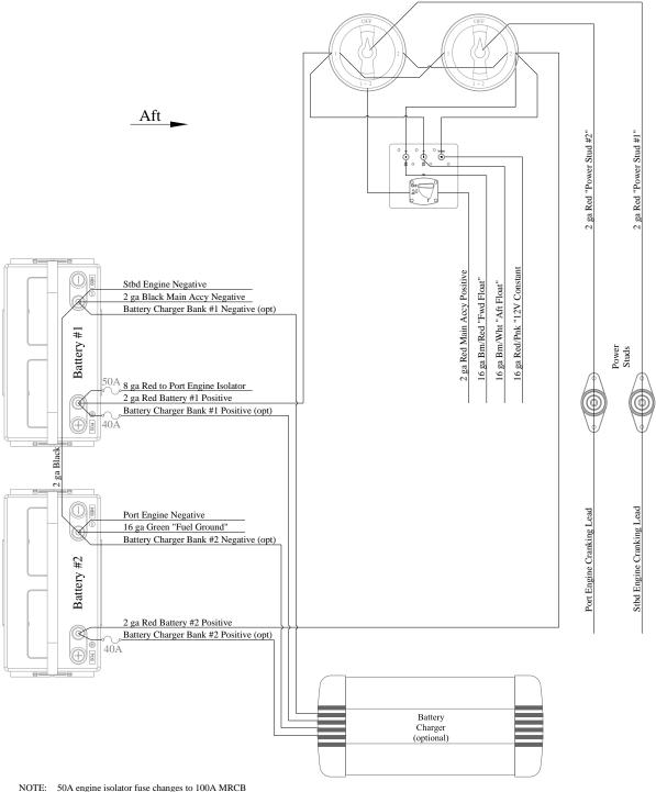
Battery Wiring with Select Switches (Dual)
