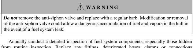
from routine inspection. Replace any fittings, deteriorated hoses, clamps or connections immediately. Fuel filter/water separators should be replaced at least annually.
