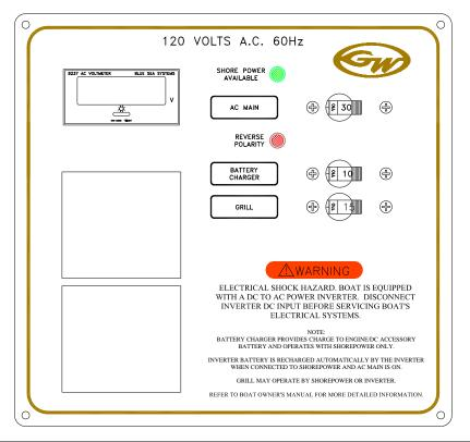
120V AC presents a high voltage shock hazard. All power supplies should be turned off and disconnected before accessing the wiring behind the AC panel. Service to the AC wiring should be performed by a qualified marine electrician.
