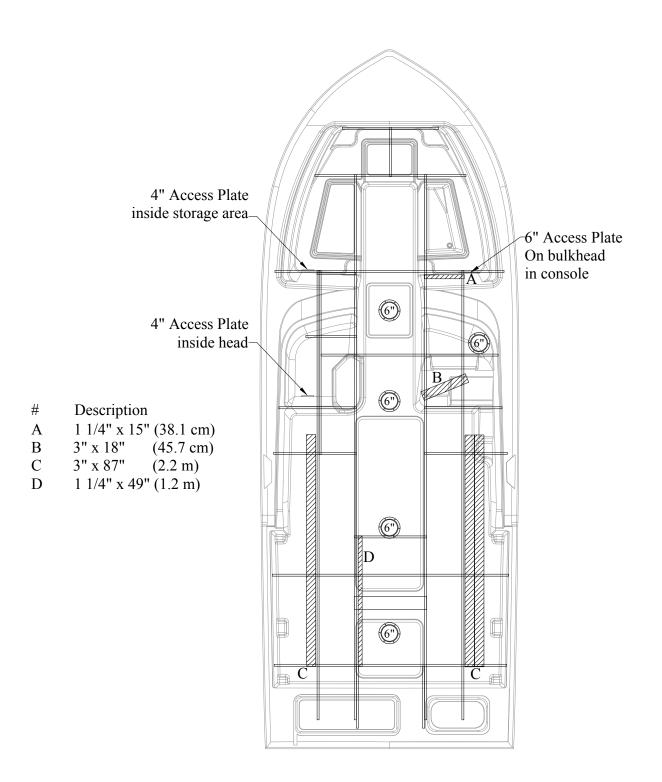
Access Plate and Rigging Tube Locations
