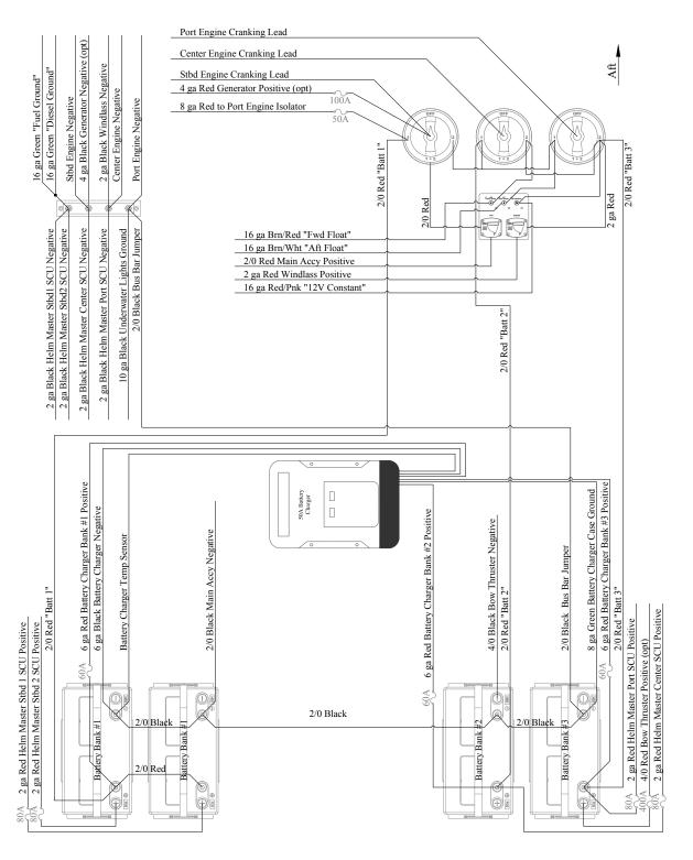
NOTE: 50A engine isolator fuse changes to 100A MRCB if the boat is equipped with V6 engines.
