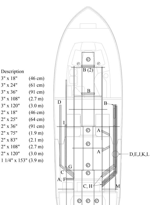
Access Plate And Rigging Tube Location
