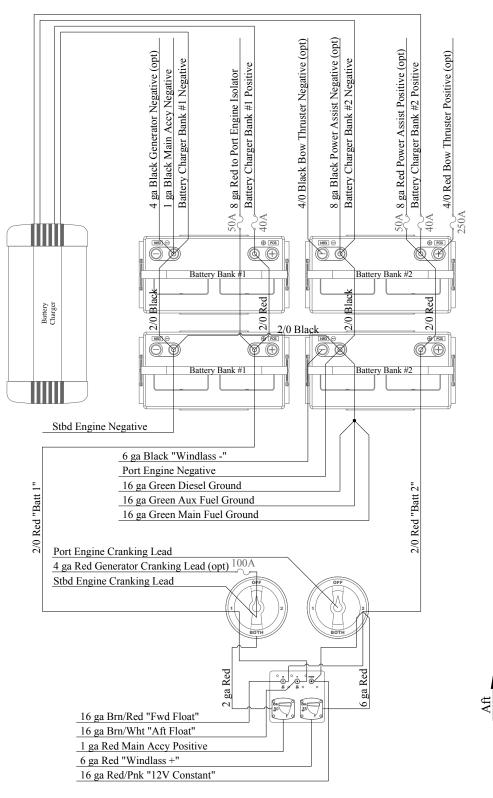
**Battery Wiring With Select Switches**
