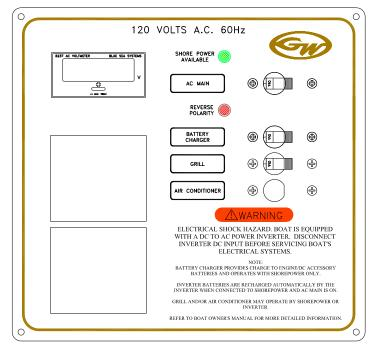
120V AC presents a high voltage shock hazard. All power supplies should be turned off and disconnected before accessing the wiring behind the AC panel. Service to the AC wiring should be performed by a qualified marine electrician.
