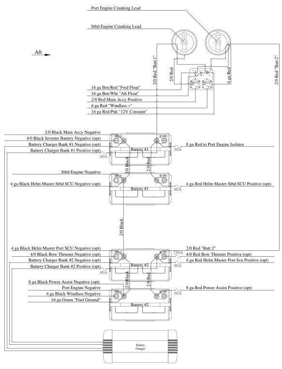
NOTE: 50A engine isolator fuse changes to 100A MRCB if the boat is equipped with V6 engines.
