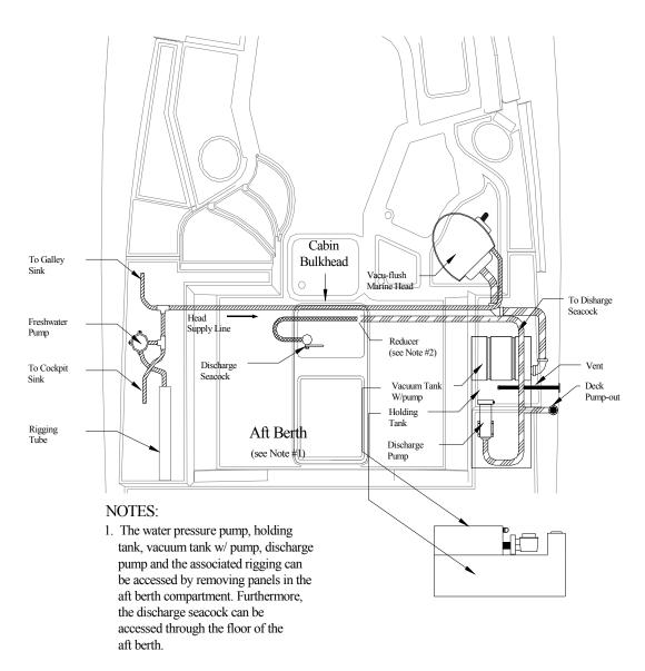
2. The discharge hose is reduced and the material is changed in the aft berth compartment.
