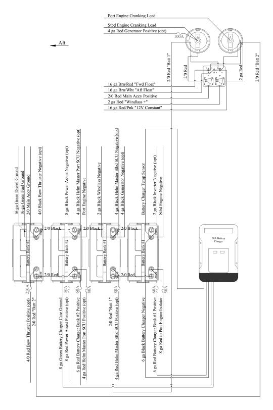
NOTE 1: Engine isolator fuse changes to 100A MRCB if the boat is powered with V6 engines.
