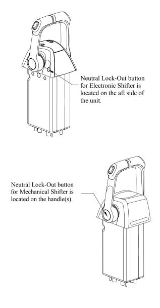
Reverse the shift mechanism to stop a boat that is moving forward. This change in direction will provide a "braking action" and slow the boat.
