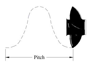
Diameter and pitch are the two basic dimensions of a propeller. Diameter is the distance across the circle made by the blade tips as the propeller rotates. Pitch is the theoretical (not accounting for slippage) forward distance the propeller would move in one revolution. An example of a propeller dimension would be 14 X 17 for a propeller having a diameter of 14" (35.6cm) and a pitch of 17" (43.8cm).
