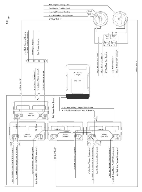
NOTE 1: 50A engine isolator fuse changes to 100A MRCB if the boat is equipped with V6 engines.
