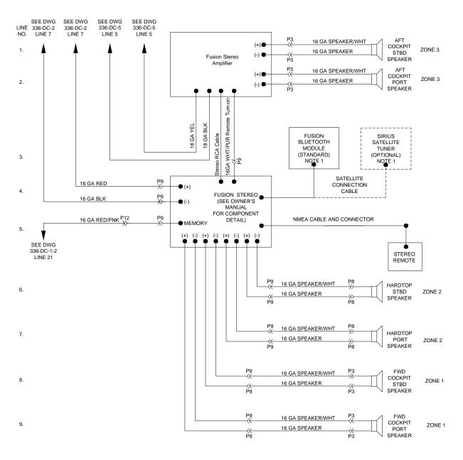
1) BLUETOOTH MODULE IS DELETED WITH SATELLITE (SAT) OPTION 2) SEE LAYOUT DRAWINGS FOR COMPONENT LOCATIONS
