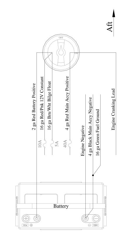
Battery Wiring With Select Switch (Standard)
