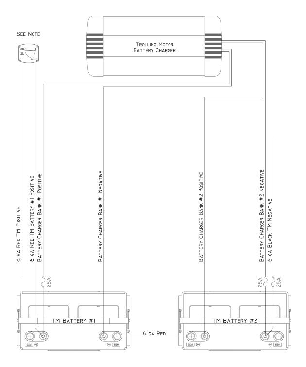
NOTE I: TROLLING MOTOR BREAKER MUST BE SIZED APPROPRIATELY FOR THE TROLLING MOTOR TO BE INSTALLED. CONSULT MANUFACTURERS INSTALLATION INSTRUCTIONS.
