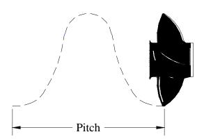
Diameter and pitch are the two basic dimensions of a propeller. Diameter is the distance across the circle made by the blade tips as the propeller rotates. Pitch is the theoretical (not accounting for slippage) forward distance the propeller would move in one revolution. An example of a propeller dimension would be 14 X 17 for a propeller having a diameter of 14" (35.6cm) and a pitch of 17" (43.8cm).
