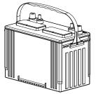
Do not allow any electrically conductive material to make contact with both the positive and negative terminals at the same time (i.e. a hand tool used when disconnecting and reconnecting battery cables). A short of this nature can cause severe burns and create dangerous sparks which could result in personal injury and/or property damage.
