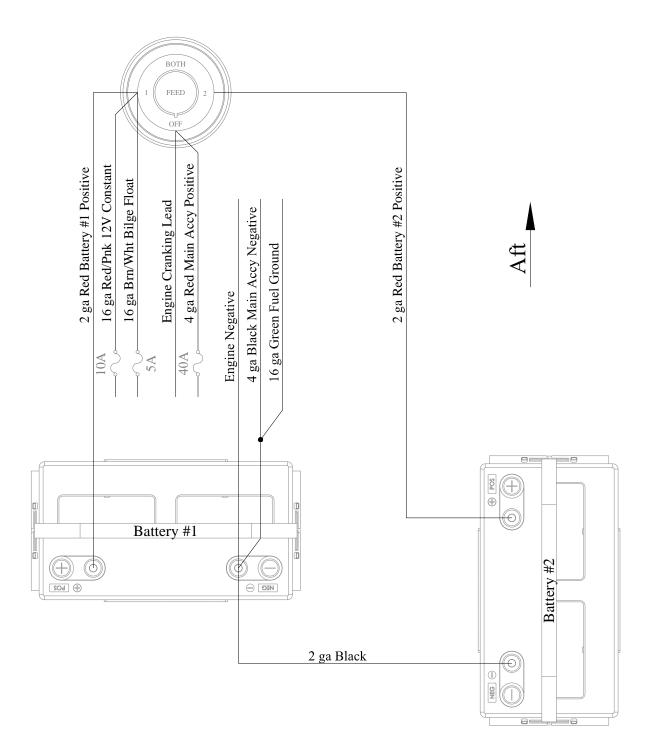
Battery Wiring with Select Switch
