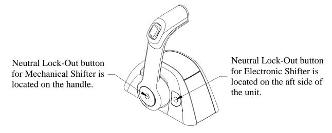
Reverse the shift mechanism to stop a boat that is moving forward. This change in direction will provide a "braking action" and slow the boat.
