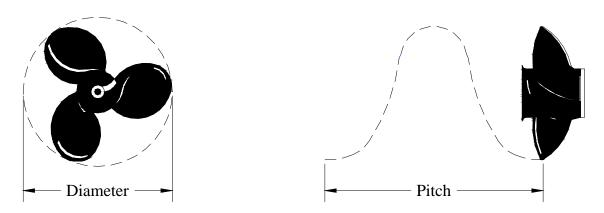
Diameter and pitch are the two basic dimensions of a propeller. Diameter is the distance across the circle made by the blade tips as the propeller rotates. Pitch is the theoretical (not accounting for slippage) forward distance the propeller would move in one revolution. An example of a propeller dimension would be 14 X 17 for a propeller having a diameter of 14" (35.6cm) and a pitch of 17" (43.8cm).
