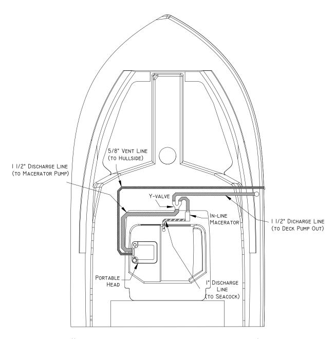
Y-VALVE IS MOUNTED HORIZONTAL ON POLY PLATE FORWARD OF CONSOLE. IT CAN BE ACCESSED THROUGH THE 6" ACCESS PLATE, NEAR FLOOR LEVEL, ON THE FORWARD CONSOLE WALL.
