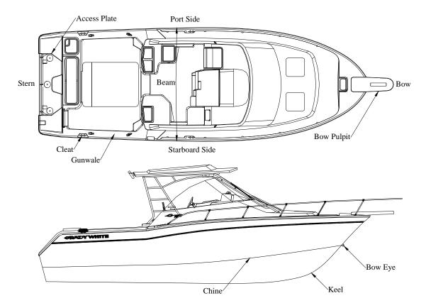
**Abeam** - a line perpendicular to a boat's keel **Access Plate** - a removable, watertight cover that provides quick entry to enclosed areas for maintenance or visual inspection
