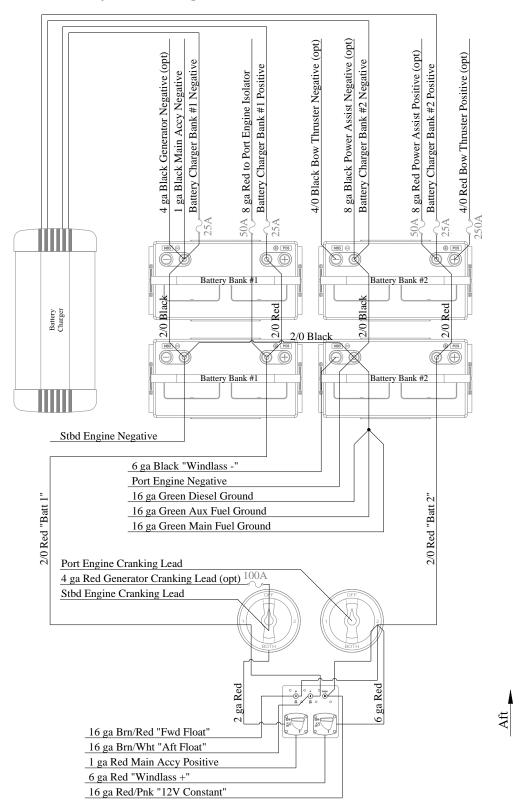
NOTE: 50A engine isolator fuse changes to 100A MRCB if the boat is equipped with V6 engines.
