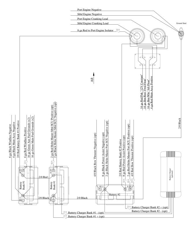
NOTE: 50A engine isolator fuse changes to 100A MRCB if the boat is equipped with V6 engines.
