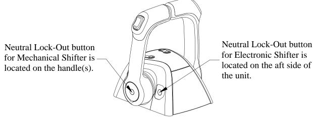
for Electronic Shifter is located on the aft side of
