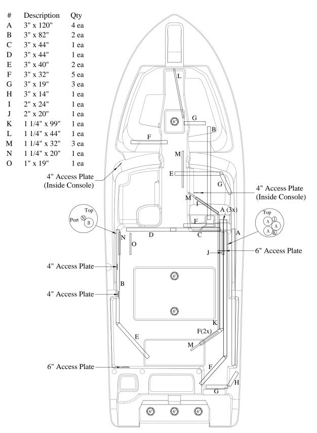
Access Plate And Rigging Tube Location
