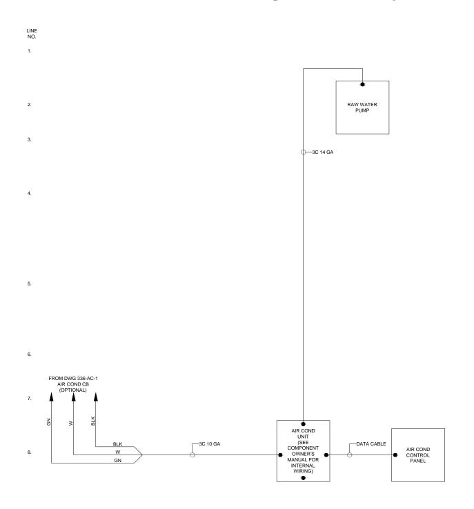
120V Air Cond. without Cockpit Cooler Diagram
