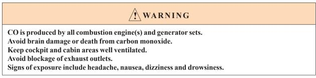
Carbon Monoxide, commonly written CO, is a colorless, odorless gas emitted from any boat's exhaust. The gas is similar in weight to the air we breathe. Therefore, it cannot be expected to rise or fall, but will accumulate in confined spaces.
