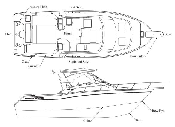
**Abeam** - a line perpendicular to a boat's keel **Access Plate** - a removable, watertight cover that provides quick entry to enclosed areas for maintenance or visual inspection
